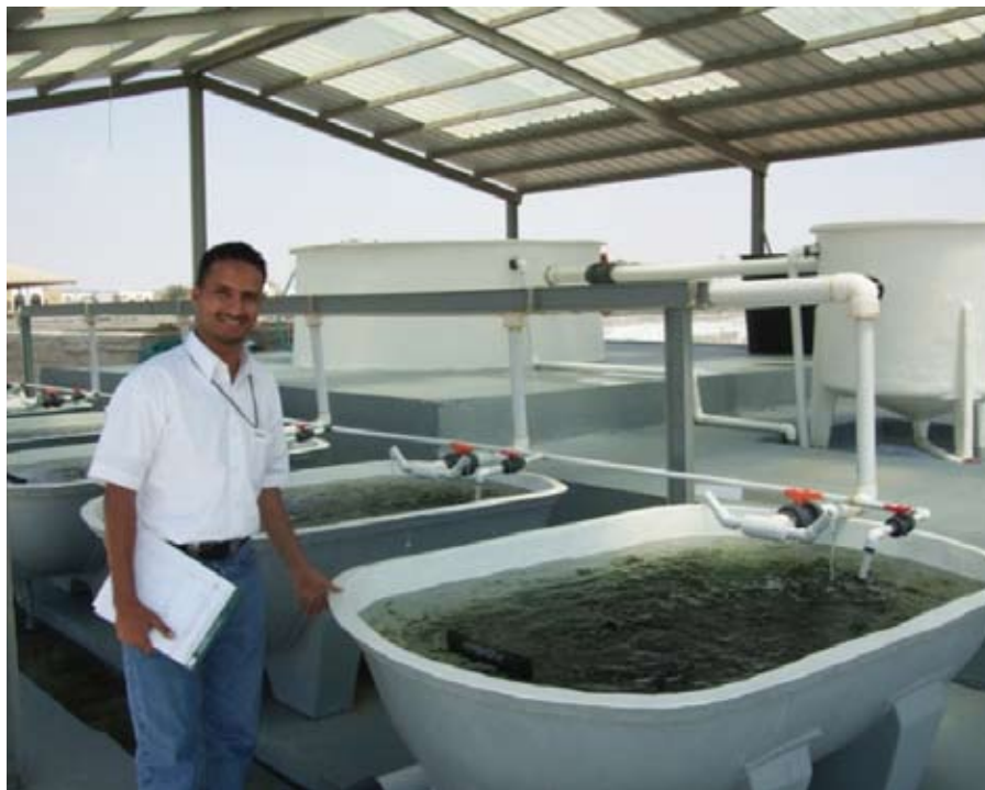
A Ministry of Agriculture project is raising tilapia in full-strength seawater in a system where seaweeds absorb nutrients from the fish effluent to allow water reuse.
