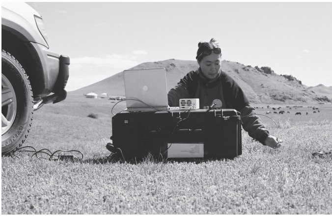
Figure 1. Portable NIRS set up for acquiring spectra in the field with hand held fiber optic probe. High Mountain Research Station, Mongolia. Photo by Doug Tolleson
