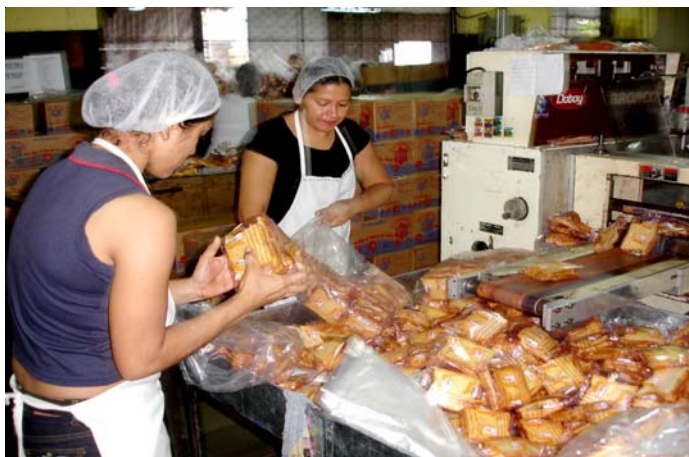
Machine wrapping of baked goods at the Pan Rey Bakery
